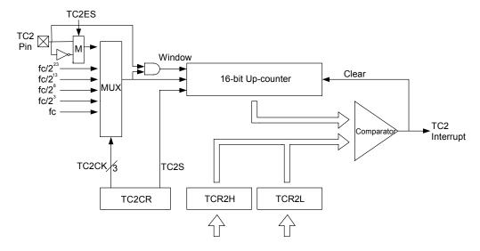
Fig 19. Configuration of Timer/Counter 2
